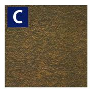
The mill scale has rusted away from the surface of the steel, due to prolonged exposure to the elements. Any remaining mill scale can be simply scraped off, and early signs of surface pitting may be visible.
