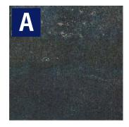
The surface of the steel is completely covered with mill scale, showing little or no signs of any rust or oxidisation, and no pitting.
