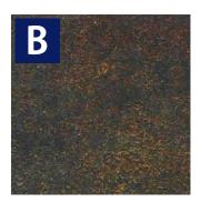
The surface of the steel has been exposed to the elements and shows signs of rusting, with the mill scale beginning to flake.
