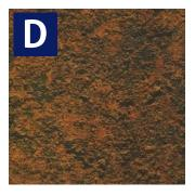
Steel surface on which the mill scale has rusted away and general pitting is visible under normal vision.
